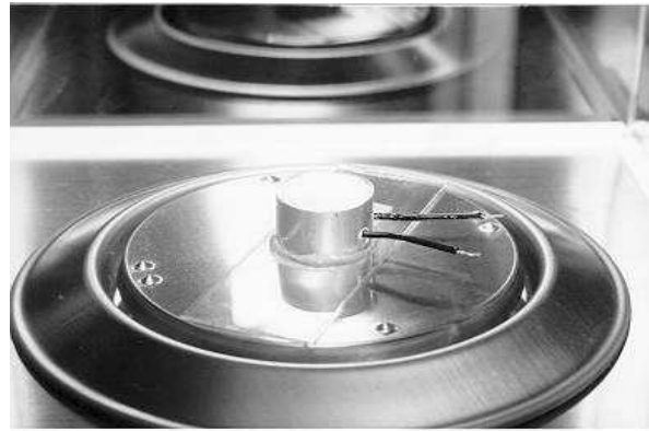
Figure 2 – Weighing of the test specimen.
